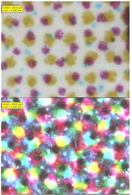
Dots in the halftones are clear and precise, as you can see more clearly in the photograph above (light part of the image); in the first picture it is also possible to see how precisely halftone dots are arranged; the same arrangement is obviously also present in the dark area, but it is more difficult to distinguish it.
