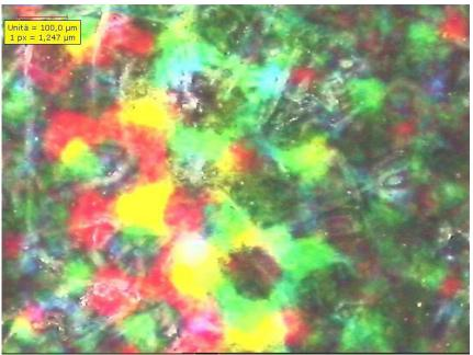
It may be noted that the halftone of the light area is clear, with more precise dots in comparison with the dots of the halftone present in the jacket and in the colour picture contained in the book.
