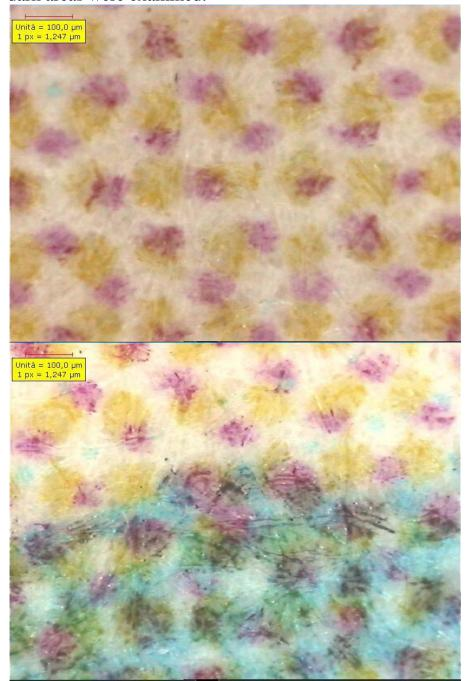
Although the cover is made of macroporous and rough cardboard, it is possible to note that halftones are precise, both in light and dark areas.
