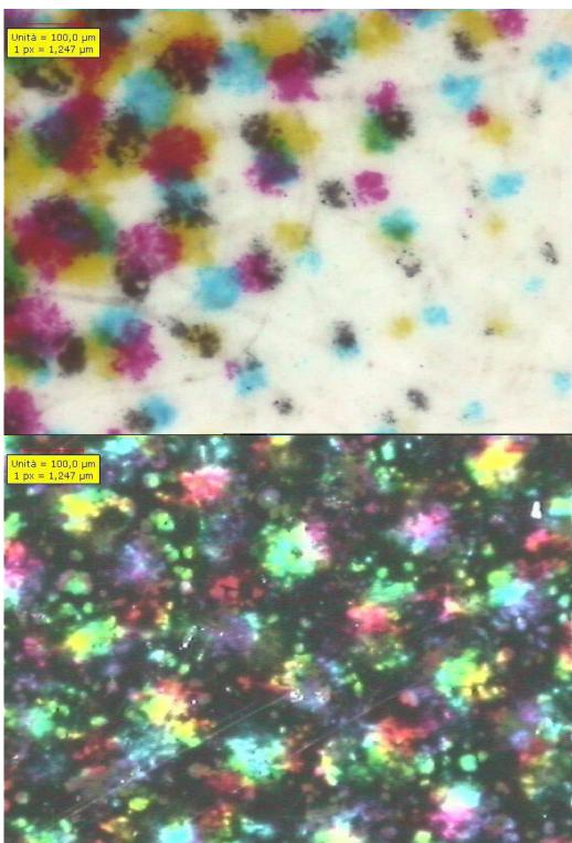
The first image shows the light dots in the photograph, the second one shows the dark dots. In both photographs, clear imperfections are evident, which are typical for printing plates (plates) incised with a chemical process.
